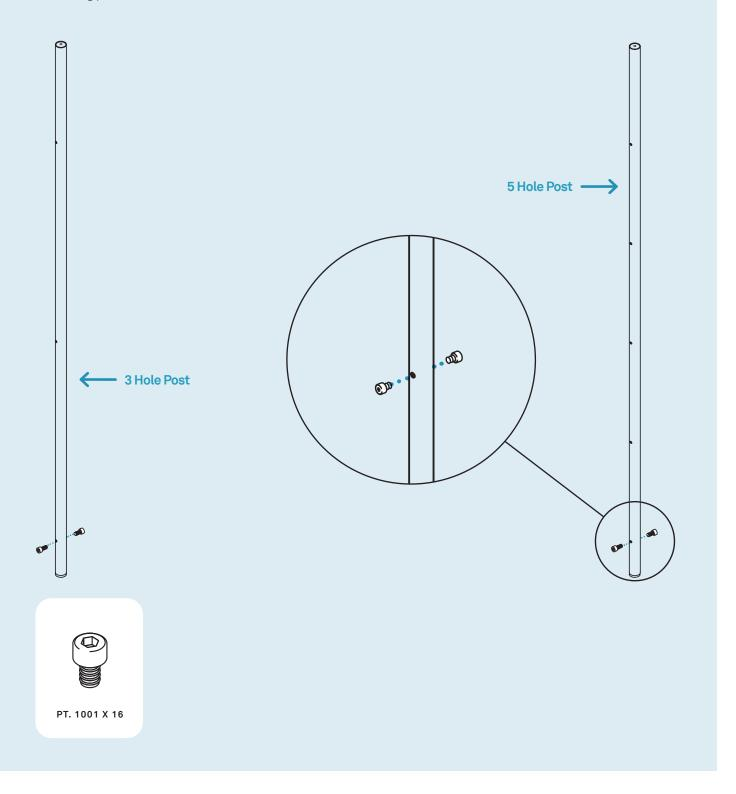
Insert post as shown. After the posts have been installed, have a second person help lift and bring the cases upright.
